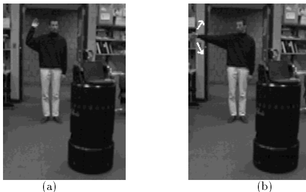
Figure 4. Example gestures: ‘Stop’ gesture (a) and ‘Follow’ gesture (b). While the ‘Stop’ gesture is a static gesture, the ‘Follow’ gesture involves motion, as indicated by the arrows.
