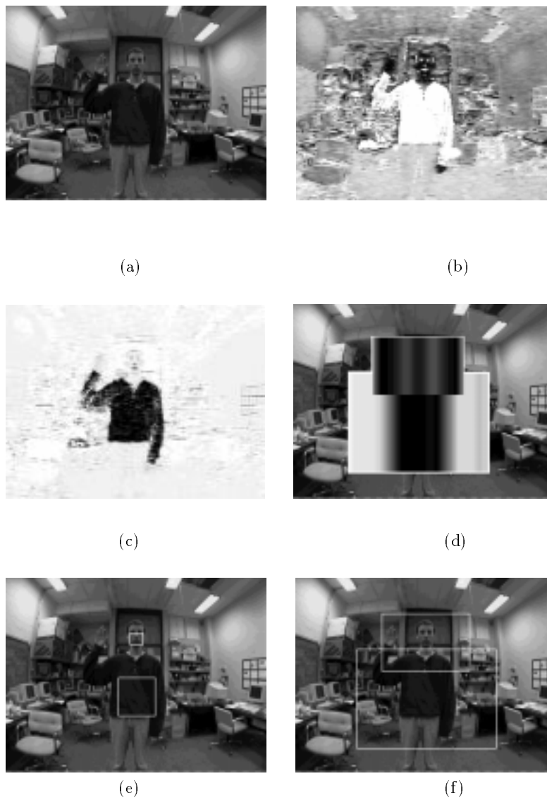
Figure 2. Tracking a person: Raw camera image (a), face-color filtered image (b) and shirt-color filtered image (c). Projection of the filtered image onto the horizontal axis (within a search window) (d). Face and shirt center, as used for tracking and adaptation of the filters (e). Search window, in which the person is expected to be found in the next image (f).
