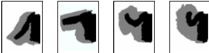
Figure 5. Examples of pose templates. The excitatory region is shown in black and the inhibitory in grey. White regions are not considered in the matching process.
