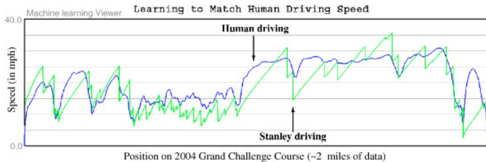
**Figure 23.** Velocity profile of a human driver and of Stanley’s velocity controller in rugged terrain. Stanley identifies controller parameters that match human driving. This plot compares human driving with Stanley’s control output.
