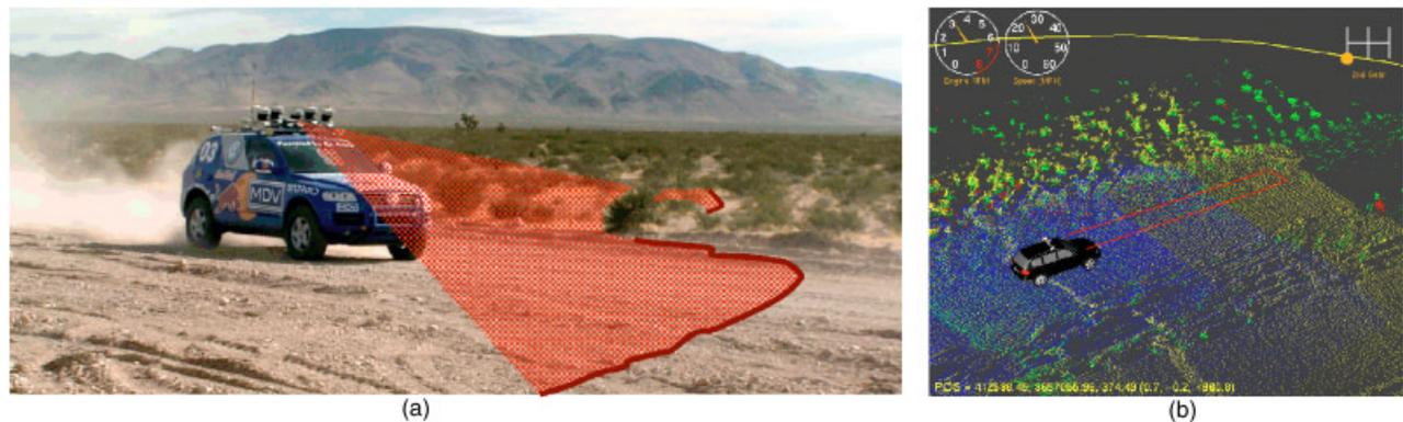
**Figure 7.** (a) Illustration of a laser sensor: The sensor is angled downward to scan the terrain in front of the vehicle as it moves. Stanley possesses five such sensors, mounted at five different angles. (b) Each laser acquires a three-dimensional (3D) point cloud over time. The point cloud is analyzed for drivable terrain and potential obstacles.
