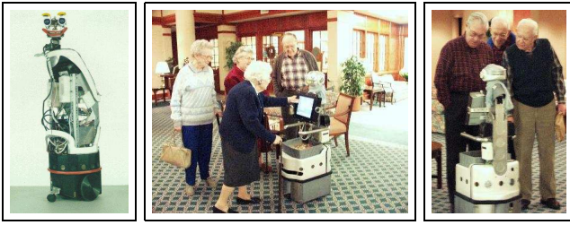
Figure 1: Nursebots Flo (left) and Pearl (center and right) interacting with elderly people during one of our field trips.
