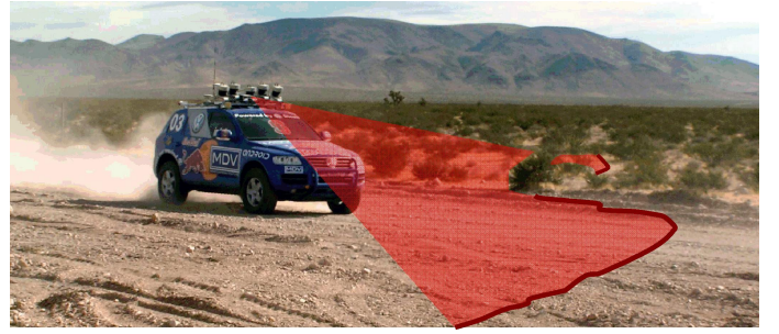
Figure 2. The vehicle uses a single line scanner to acquire surface data from the terrain to make driving decisions.
