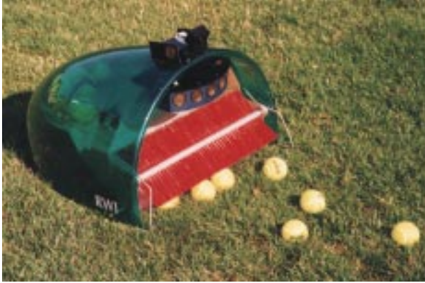
Figure 1: Jeeves, an entry from Carnegie Mellon University. A large rotating brush lifts tennis balls into a ramp inside the robot's shell. To unload balls, Jeeves can reverse the direction of the brush. Jeeves moves approximately 60 cm/sec. When equipped with a basket, Jeeves can hold approximately 100 balls—sufficiently many for a real tennis court.
