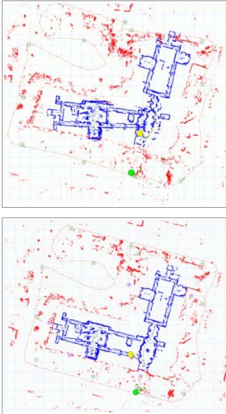
Fig. 6. Indoor mapping. Top: just based on the IMU and SLAM. Bottom: factoring in GPS data acquired outdoors. This experiment highlights the utility of our hybrid SLAM algorithm that factors in GPS measurements as available.
