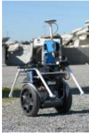
Fig. 4. The Segbot, a robot based on the Segway RMP platform and developed through the DARPA MARS program.
