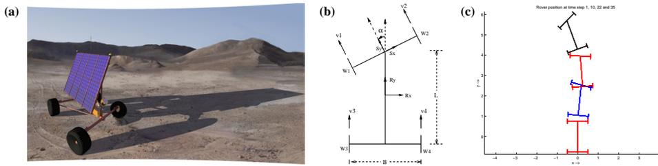
**Figure 3:** (a) The Hyperion rover, a mobile robot being developed at CMU. (b) Kinematic model. (c) Rover position at time step 1, 10, 22 and 35.
