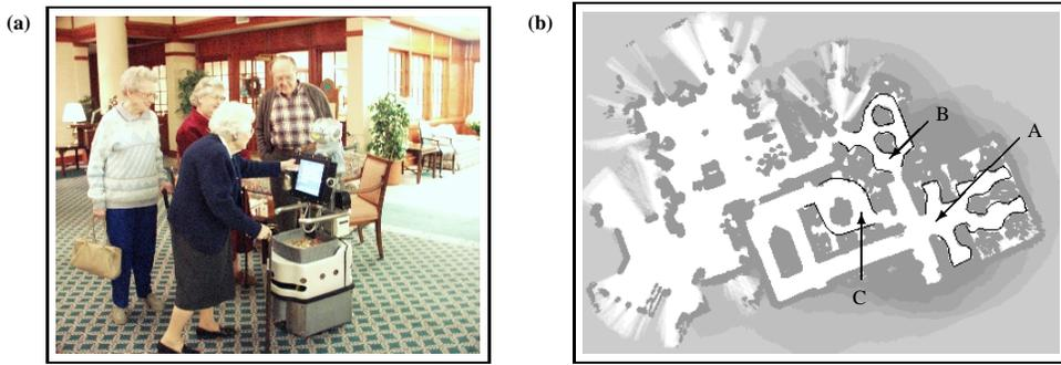
**Figure 1:** (a) Robot Pearl, as it interacts with elderly people at an assisted living facility in Oakmont, PA. (b) Occupancy grid map. Shown here are also three testing locations labeled A, B, and C, and regions of high costs (black contours).
