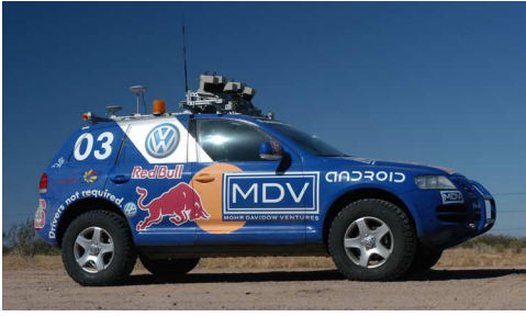
Figure 1: Stanley won the 2005 DARPA Grand Challenge by completing a 132 mile desert route in just under 7 hours. The algorithm described in this paper was the deciding factor in Stanley’s speed for nearly 20% of the race – more than any other constraint except the DARPA-imposed speed limits.
