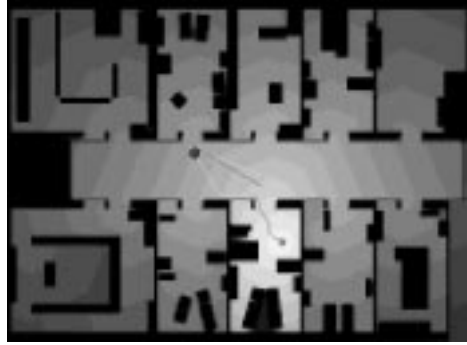
Figure 2. The path planner computes the optimal path to goal position (marked by 0) and the next intermediate goal position which is sent to the collision avoidance.
