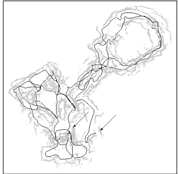
Figure 13: The map of the Smithsonian, generated with corrected position estimates, from correction parameters computed in the Carnegie Museum. Again the arrows correspond to the same point in the museum.
