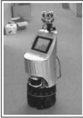
**Figure 1:** *Florence Nightingale*, the prototype nursing home robot used in these experiments.
