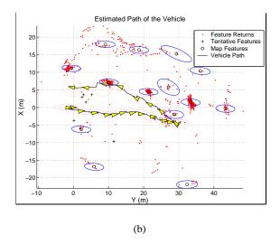
Figure 3: (a) 3D volumetric map, acquired by a mobile robot in real-time. The lower part of the map is below the robot's sensors, hence is not modeled. (b) Map of underwater landmarks, acquired by the submersible vehicle Oberon at the University of Sydney. Courtesy of Stefan Williams and Hugh Durrant-Whyte.
