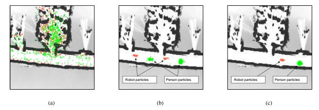
Figure 2: Evolution of the conditional particle filter from global uncertainty to successful localization and tracking.
