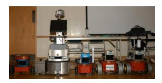
**Figure 1**: The CMU laser tag system consists of six robots based on Pioneer and Scout platforms, of which five are shown here. The robots are equipped with infrared emitters and detectors. Navigation is achieved using the CARMEN software system (Montemerlo et al., 2002).
