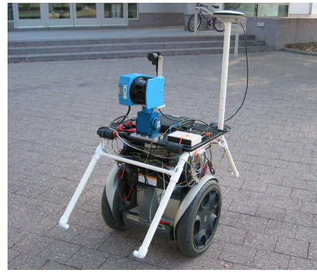
Figure 3: The robotic vehicle is based on a Segway RMP, equipped with a vertically oriented SICK laser range finder mounted on an Amtec pan/tilt unit. The robot uses a highly tuned Inertial Measurement Unit and a GPS for localization.
