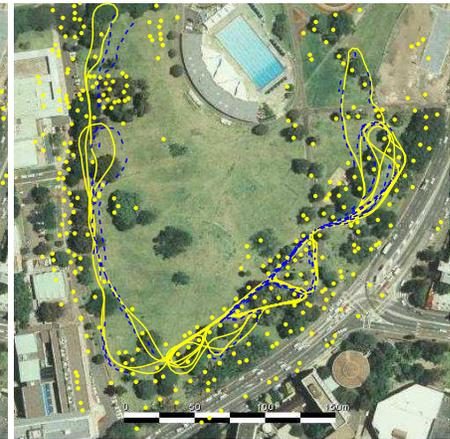
**Figure 1:** FastSLAM 2.0 applied to the Victoria Park benchmark data set using only  $M=1$  particle. The accuracy of the recovered path and the resulting map is indistinguishable from that the best EKF-style methods and the original FastSLAM algorithm with  $M=100$  particles.
