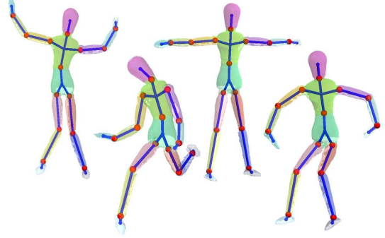
Figure 3: Four different poses from the puppet dataset display the 15 rigid parts and the articulated skeleton, both of which are recovered automatically
