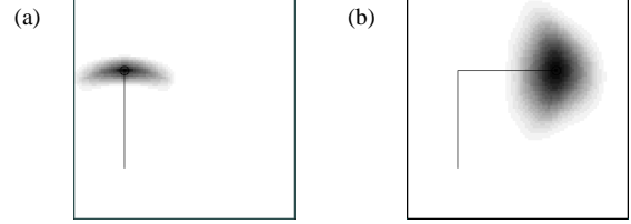
Figure 2: Probabilistic model of robot motion: Accumulated uncertainty after moving (a) 40 meter, (b) 80 meter.
