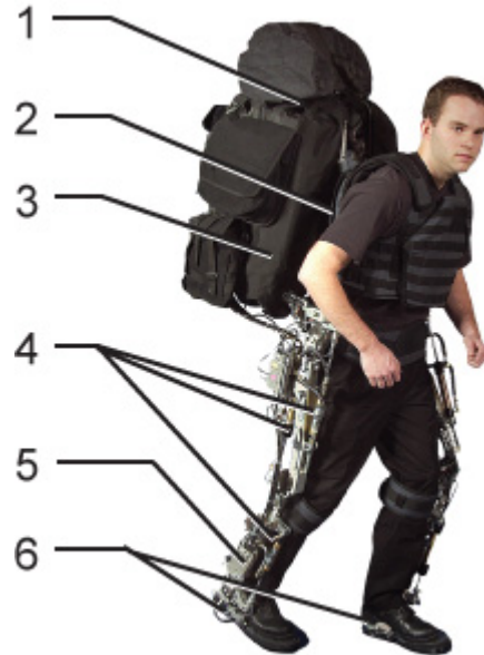
Fig. 1. Berkeley Lower Extremity Exoskeleton (BLEEX) first generation prototype and pilot. 1: Hydraulic power supply and payload occupy the upper portion of the backpack; 2: Rigid BLEEX spine connected to the flexible pilot vest; 3: Central control computer occupies the lower portion of the backpack; 4: Some of the hydraulic actuators (ankle, knee and hip); 5: Two of the control network's Remote I/O Modules (RIOM); 6: Rigid connection of the BLEEX feet to the pilot's boots. More photographs can be found at http://bleex.me.berkeley.edu
