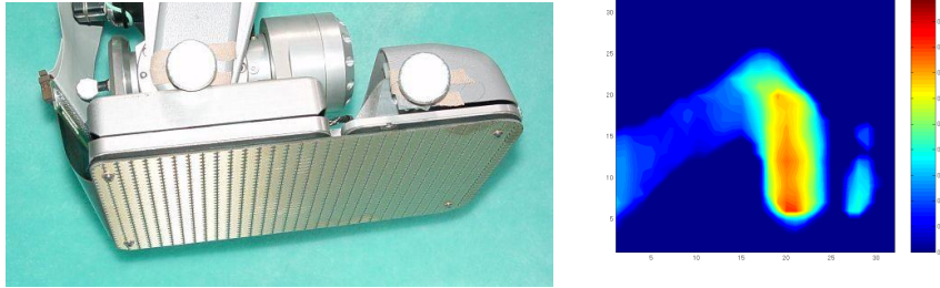
Fig. 6. Humanoid robot foot with pressure sensor grid and human foot pressure result
