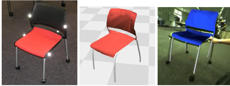
Fig. 8. (a) Real chair with retroreflective markers illuminated. (b) 3D model of chair as recovered by a laser scanner. (c) Virtual chair is overlaid in real-time. Both the chair and the camera are in motion.
