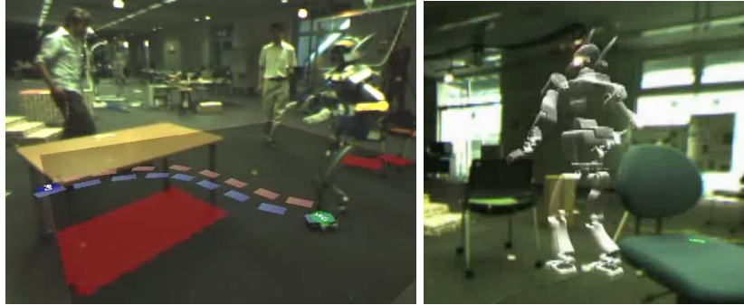
Fig. 10. Augmenting reality for visualization of planning and execution. (a) Footstep plan displayed onto the world. (b) Augmented reality with a simulated robot amongst real obstacles.
