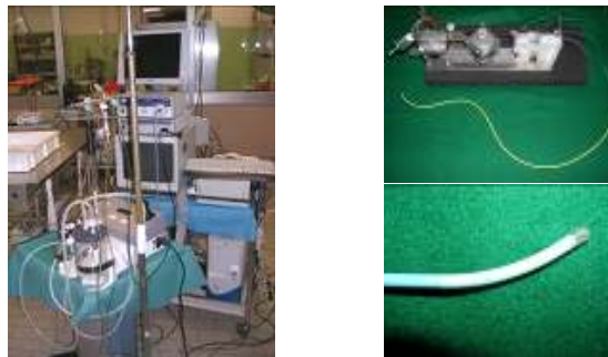
Fig. 6. On the left the robot-assisted endoscopic platform is set in the operating room; on the right, from top to bottom, the motor unit and the steerable catheter tip are shown.
