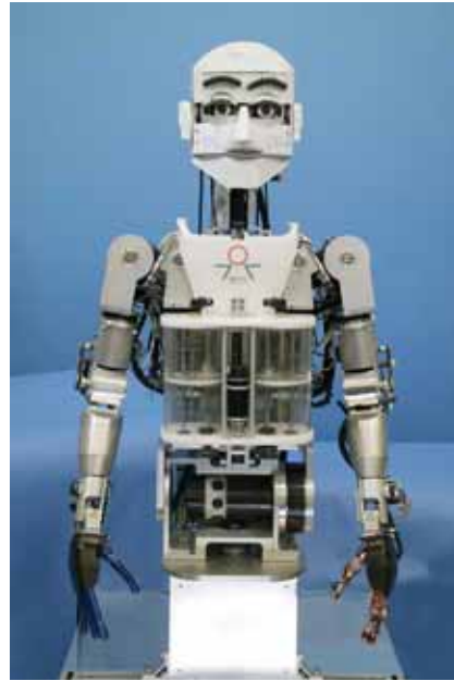
Fig. 2 Emotion Expression Humanoid Robot WE-4RII
