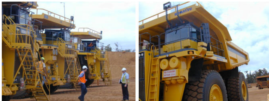
Fig. 11. Truck fleet and a truck retrofitted with a laser based tracking system
