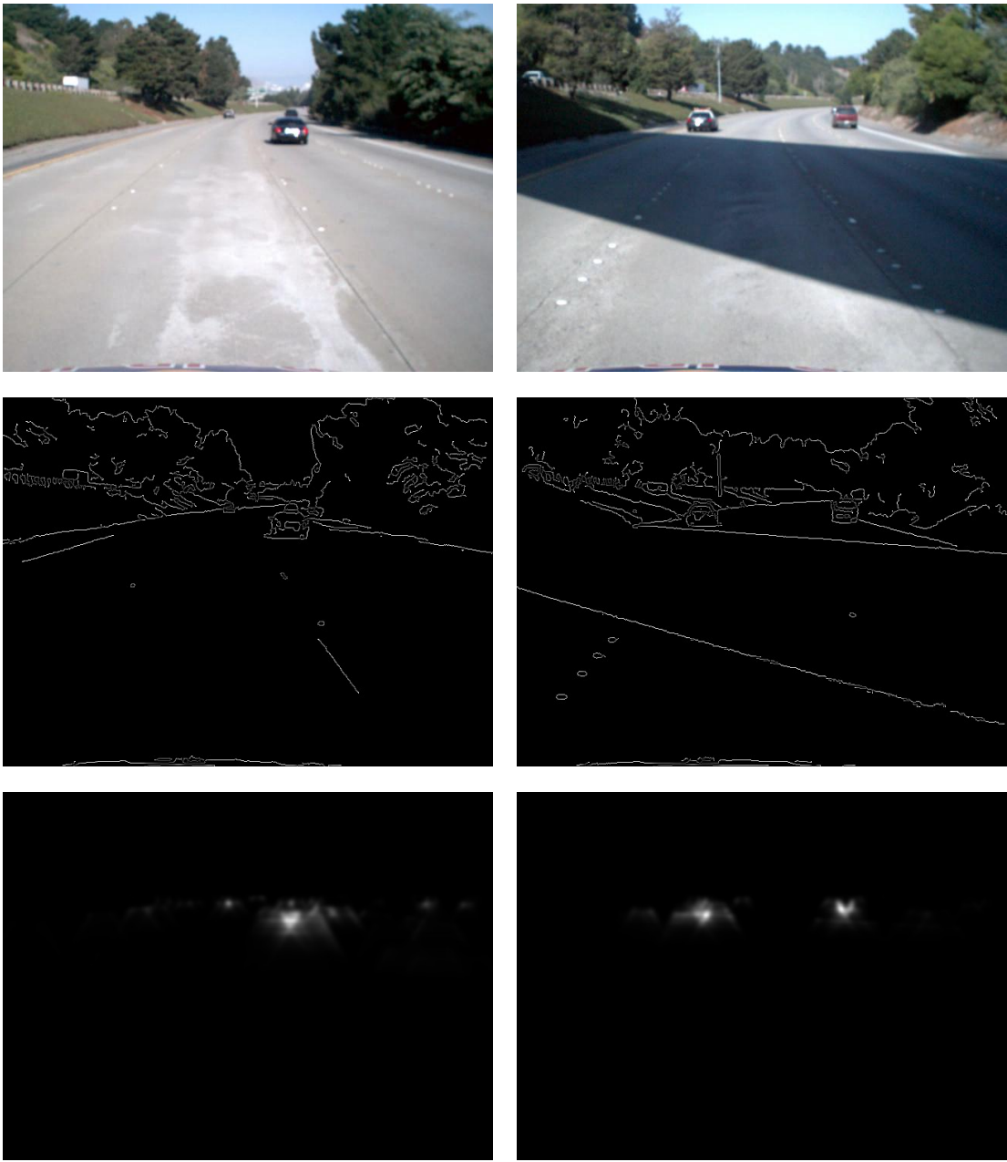
Figure 3: Response of edge pattern, with scale invariance applied through use of estimated range of car sizes for each scanline.
