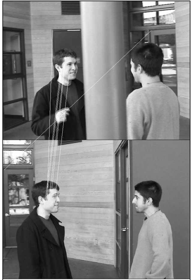
Figure 4: SIFT performs well when matching features across object rotation in depth at video resolution.
