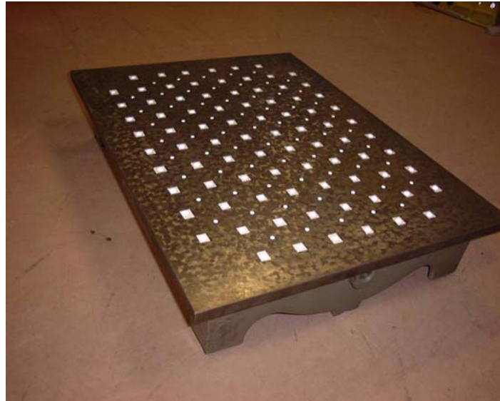
Figure 5.19. Image of the surface plate with the high intensity targets (on the white paper squares) and the low intensity targets (circular targets)
