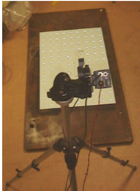
Figure 4.19. Arrangement of the target test field and camera
